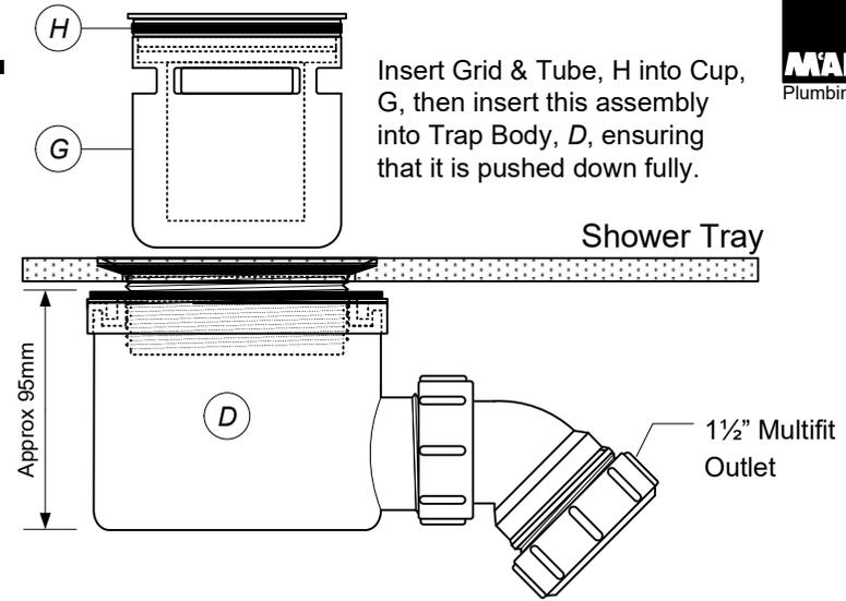
Insert Grid & Tube, H into Cup, G, then insert this assembly into Trap Body, D, ensuring that it is pushed down fully.
